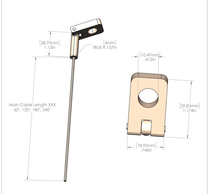
3/32" 7 x 7 Galvanized Swiveling Eye End Cable Cable End mount will Rotate 180 Degrees Safe Working Load 154 Lbs
