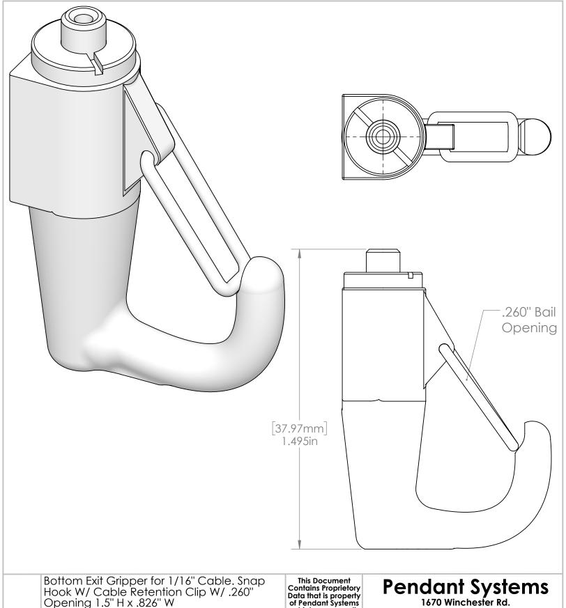
Bottom Exit Gripper for 1/16" Cable. Snap Hook W/ Cable Retention Clip W/ .260" Opening 1.5" H x .826" W
