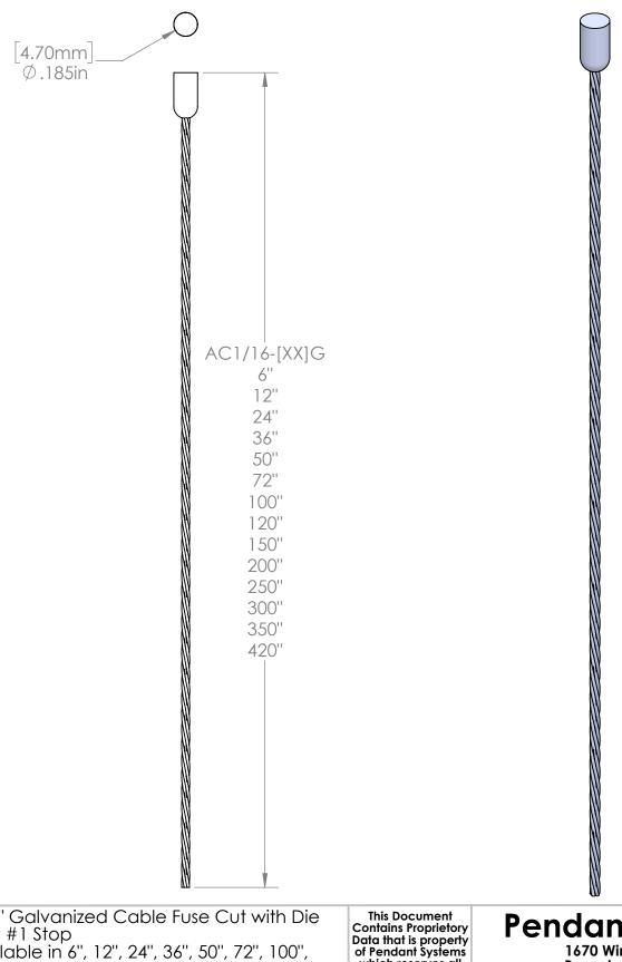
1/16" Galvanized Cable Fuse Cut with Die Cast #1 Stop Available in 6", 12", 24", 36", 50", 72", 100", 120", 150", 200", 250", 300", 350", & 420" Lengths 7x7 Cable - MAX LOAD 480 lbs
